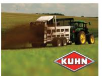
VertiSpread® vertical beaters, is designed to haul and spread solid materials from dairies and feedlots, including gutter manure, yard scrapings, bedding pack and feedlot manure. The hydraulic push-type design means no apron chains, fewer moving parts and dependable service life. www.kuhn.com.
