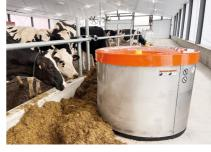
pushes silage or hay to the animal to increase their daily consumption. With its large drum and superior pushing force, it can handle wider and heavier feed lines. The robot is easily controlled using a tablet.
